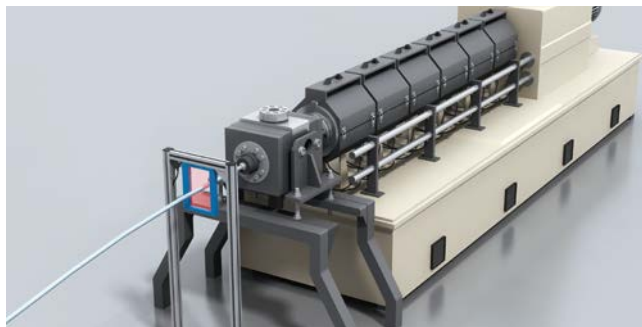
Quality control for cutting processes through automated 100 % length measurement directly on the material and efficient statistical process control.
